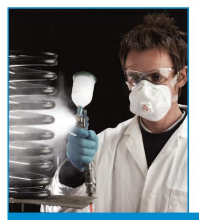
**5** All electrostatic equipment that is in contact with the VICOTE powder must be thoroughly stripped and cleaned to remove all vestiges of previously used powders. Powder delivery hoses should be dedicated to VICOTE Coatings unless they can be completely cleaned of other powders. Guns should be completely stripped down and ideally washed with (for example) IPA and then dried. If this step is not undertaken the finished coating may contain significant surface defects.
